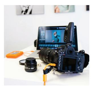
Finally, I connected my Nikon D750 with the Nikkor 70-200mm lens directly to the computer using the 15' Tether Tools TetherPro USB 2.0 Mini-B 8-Pin Cable and shot tethered straight into Lightroom so I could see exactly what the shoot was looking like in close detail.
