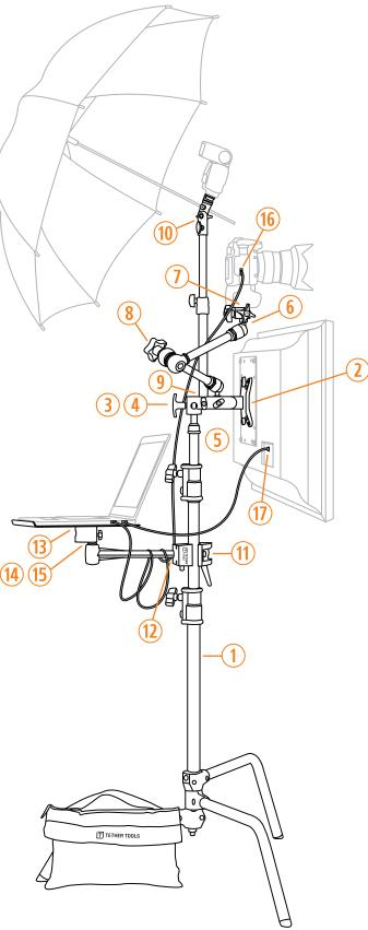
Place the Dual Wina Sand Baa on the back stand lea that is perpendicular to the monitor. \*A SecureStrap is recommended to fasten your laptop computer to your Tether Table Aero, insuring it will stay firmly in place.
